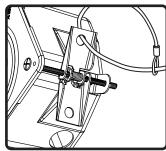
**6.** If required, attach seismic restraint system to the hole in the metal clamping arm, then to reinforced structure (safety cable not included).
